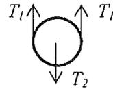
$$2.T_1 - T_2 - P_{polea} = M_{polea} \cdot a \rightarrow 2.T_1 = T_2$$
