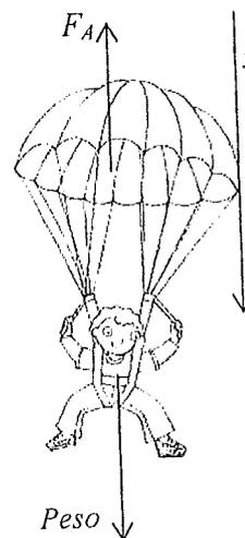
$$P - F_A = m.a \xrightarrow{\text{despejo}} a = \frac{m.g}{m} - \frac{k.v}{m} \xrightarrow{\text{simplifico}} a = 10 - 2.v$$
